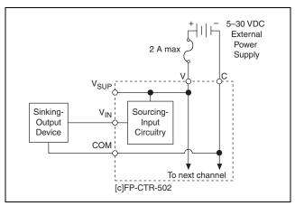
Figure 3. Wiring a Count-Input or Gate-Input Channel to a Sinking-Output Device
